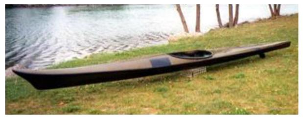
The newest of the Wave series of kayaks, the under-water section of the bow has been sharpened from the Wave Excel and given added flare above the waterline for a faster ride and for riding up over the waves. The enhanced underwater forebody also reduces drag and provides additional buoyancy over the Wave Excel in rougher water.
